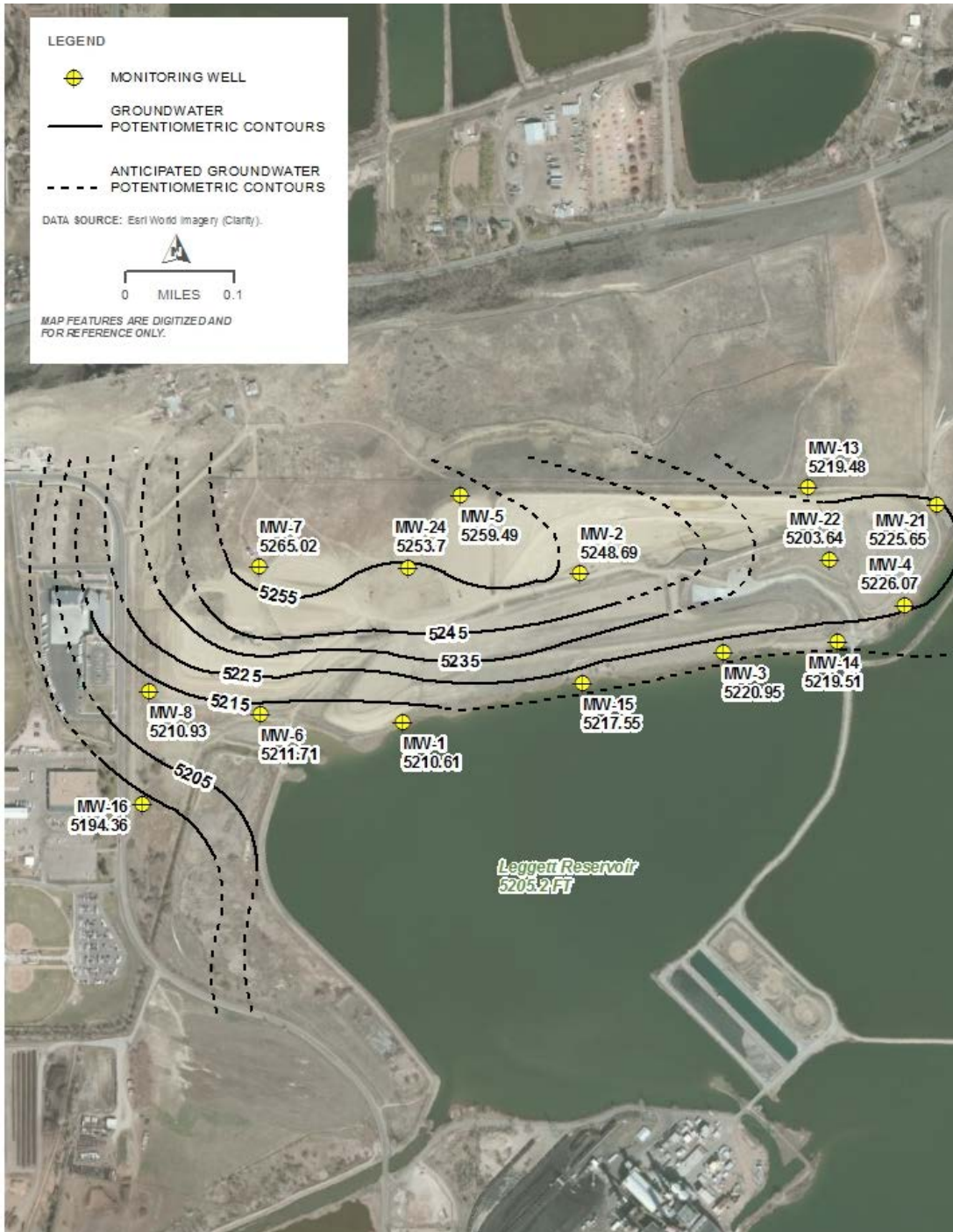
Figure 3.2-3. Valmont Station Potentiometric Surface
