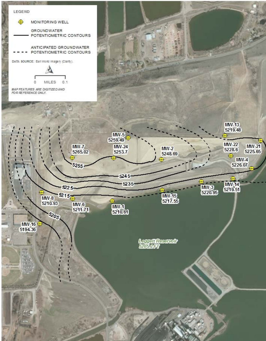
Figure 5.4-1. Valmont Site Water Level Contours
